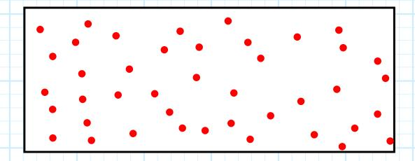
However, since these particles posses thermal energy (i.e., heat) they are moving randomly. As a result, at some later time, the particles have all moved, but are still uniformly distributed throughout the volume:
