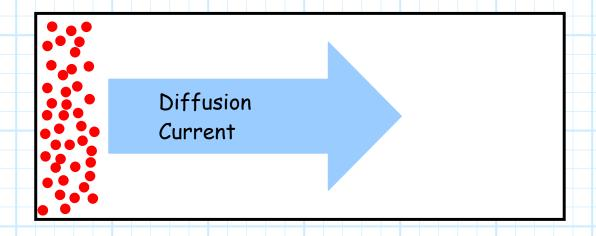
Current generated by this mechanism is referred to as **Diffusion Current**.
